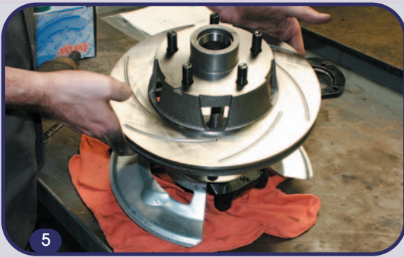
5. The rotor and hub assembly is placed on the spindle as shown.
