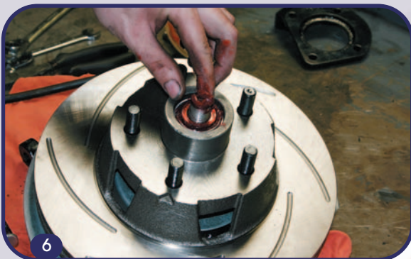
6. Pack and install the outer wheel bearing. Make sure you grease every square inch of that bearing and the top of the spindle.
