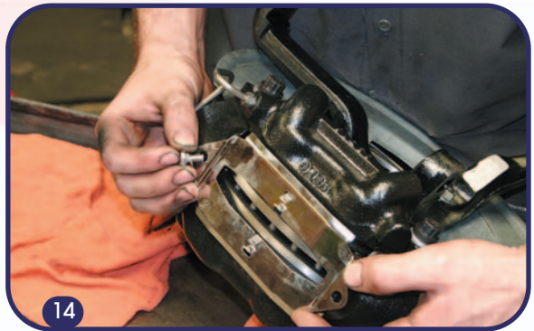
14. Install the stainless steel retaining splash shield and secure with the retaining bolts and lock washers as shown. Torque to approx. 7-11 ft.-lbs.
