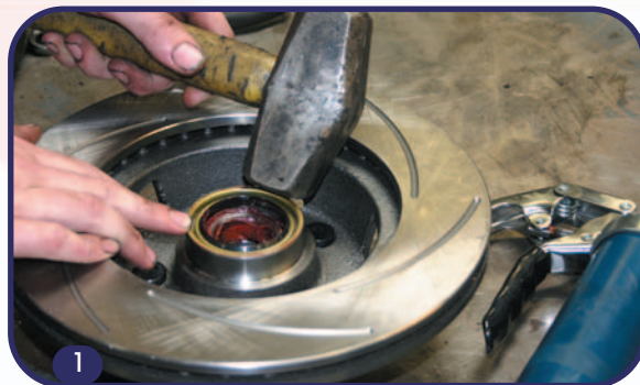
1. Here, we've taken our freshly-lubed inner bearing (the larger of the two) and placed it in the center "cup" of the rotor assembly. Then, we've applied more grease under the seal, and gently tapped it home.
