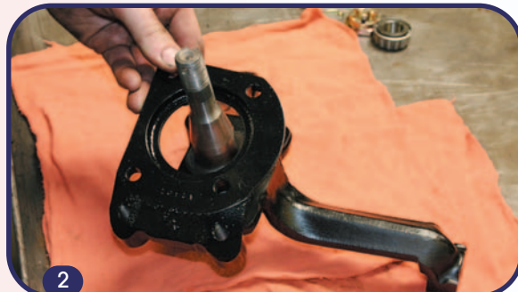
2. Check out those freshly de-greased and painted spindles! Yep, those are Old Glory originals, believe it or not. If you read our front end rebuild story, you'll see that we've totally removed our old spindles... Here, we're positioning the caliper mounting bracket. You'll need to make sure the mounting bracket bosses face towards the inside of the car. The brackets are marked right or left.
