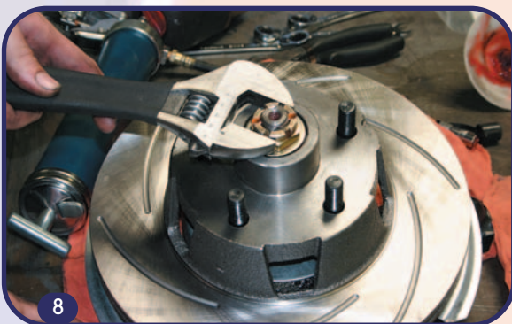
8. Here we're tightening the spindle nut. The procedure is described in detail in the kit instructions (and should be followed to the letter), but essentially the rotor should be rotated while the spindle nut is tightened (torqued to approx. 17-25 ft.-lbs.). The nut is then backed off 1/2 turn and retightened to 10-15 ft.-lbs. The nut should be positioned so that a set of slots are in line with the cotter pin hole.
