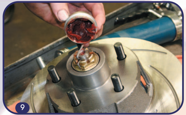
9. As per the photo, the cotter pin is inserted and bent. The grease cap should be packed (with you know what) and positioned.
