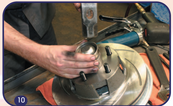
10. We temporarily place a spacer over the grease cap and gently tap until it's secure. How many dented grease caps have you seen before?
