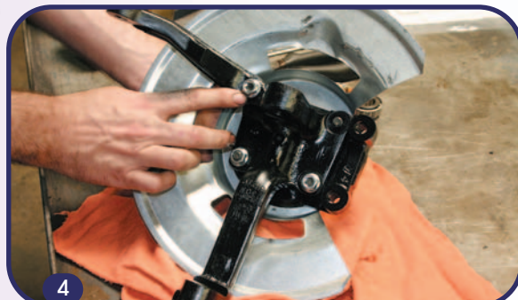
4. Secure the shield and bracket to the spindle with the grade 8 bolts provided in the kit. Note that the heads of the bolts are on the outside. Then tighten the locknuts (torque to 35-45 ft.-lbs.).
