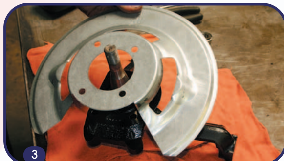
3. Next is the placement of the rotor splash shield. Like the brackets, these are marked right or left. The "hole" in the shield is where the caliper assembly will fit. Note that they must face the front of the car.
