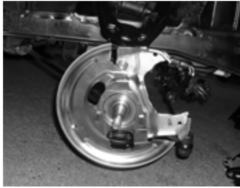
The bracket and the shield were installed with the bolts supplied and secured with the tab locks on the splash shield.
